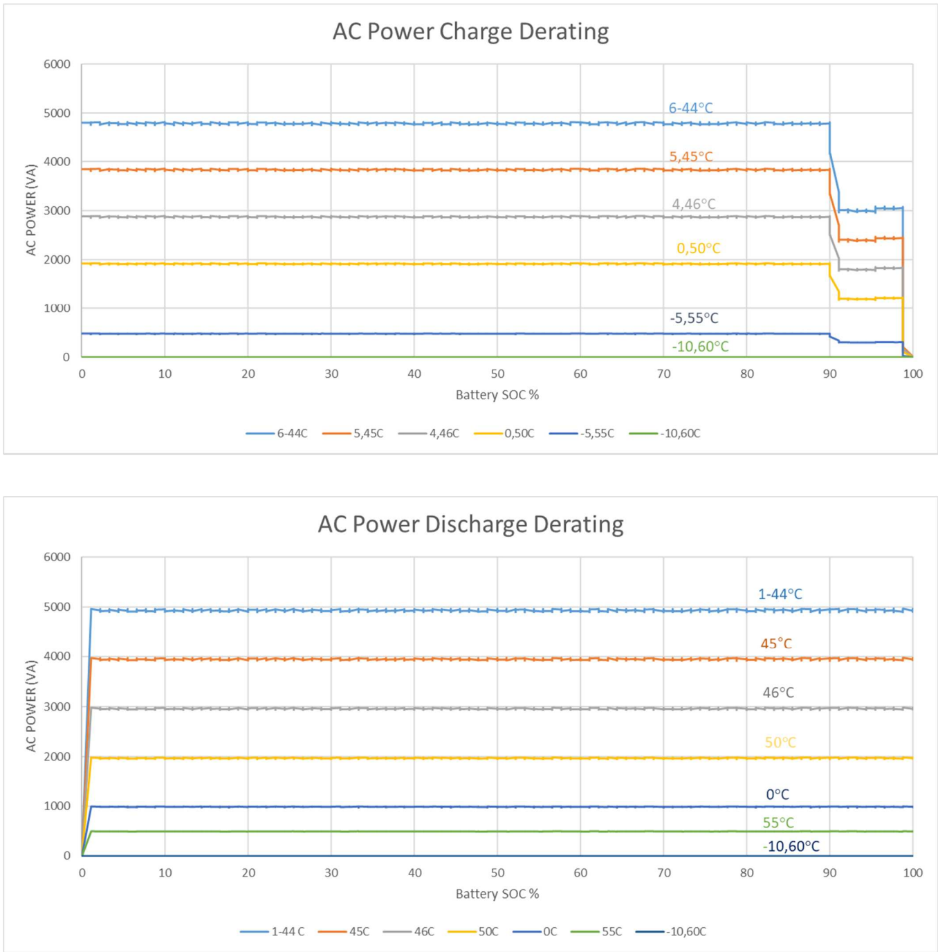
Figure 21: Energy storage system thermal derated charge and discharge curves with base battery cabinet including four Pylontech US3000C modules.
