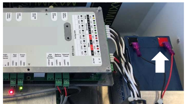
Figure 21: Connecting the AGM battery after permission to operate.
